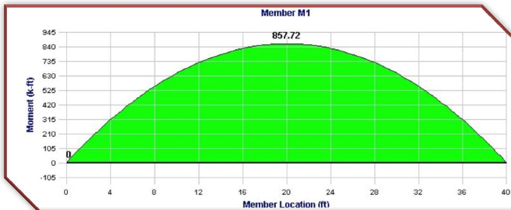
Figure 23: Maximum Moment on Interior Ledger Beam
